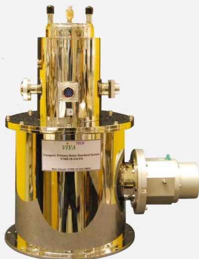
Figure 2 Cryostat Blackbody with Replaceable Feed-horn Assembly
