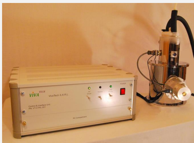
Figure 3 Controller (PC stowed) with Cryostat in Auto-Fill Operation (Cold)
